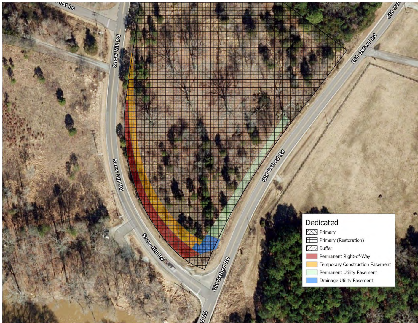
Figure 5 NCDOT Easement Request at Eno River Diabase Sill Preserve
